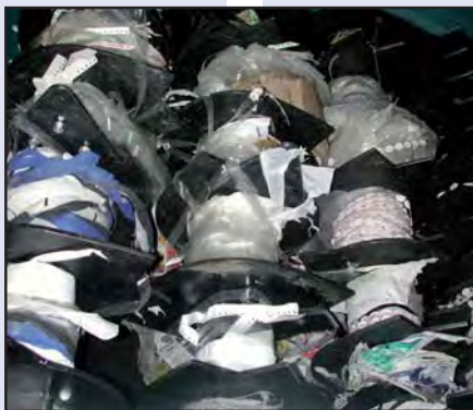
Screen clogged with plastic bags at Recycling Centre
