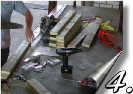
If using a handsaw and chisel, cut  $\frac{3}{4}$  in. down at the 3- $\frac{1}{2}$  in. line. Then cut a  $\frac{1}{2}$  in. deep groove into the end of the board. Place a thick wood chisel in the end groove and split the wood with a hammer to the 3- $\frac{1}{2}$  in. cut.
