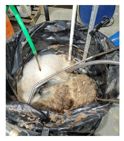
Photo 2: Feed Tank with Foam During Operation
