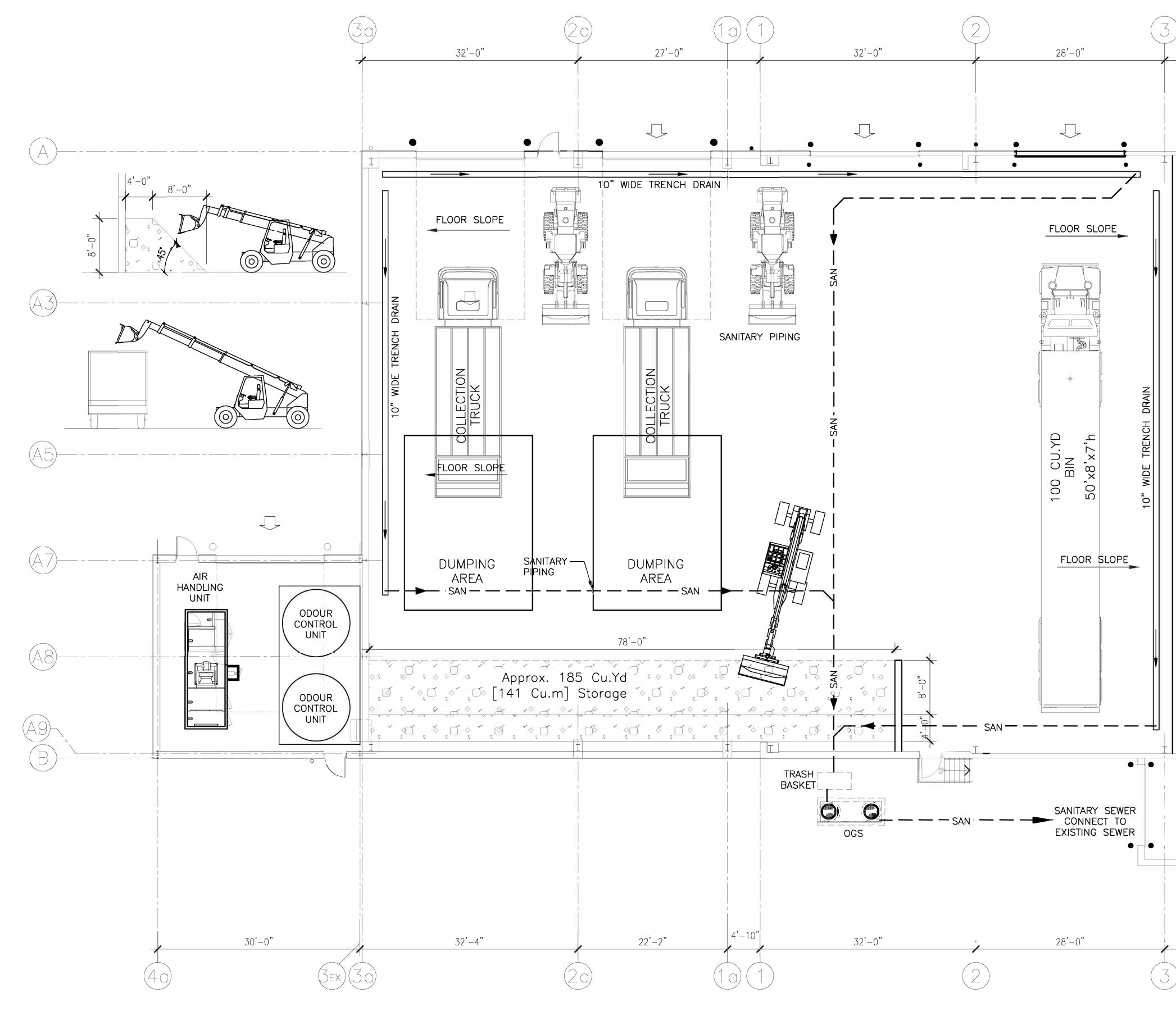
PARTIAL FIBRE RECYCLING BUILDING PLAN SCALE: 1/8" = 1'-0"
