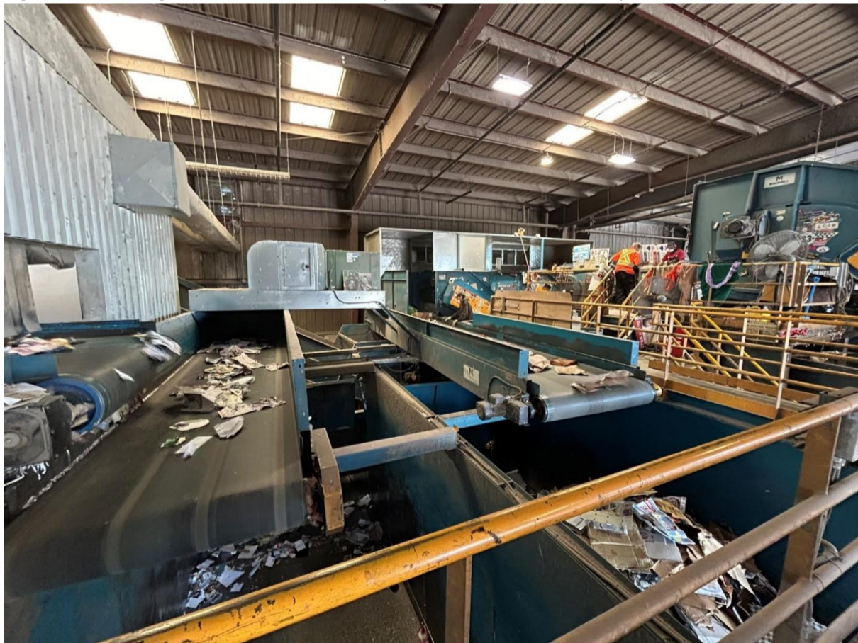
Fig 2.19 –Left to right: Sort room, final conveyors, screen, and sort conveyor (C3)
